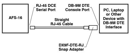
Figure 4.2: Connecting DB-9M DTE Devices to the AFS Control Module's Serial Port
